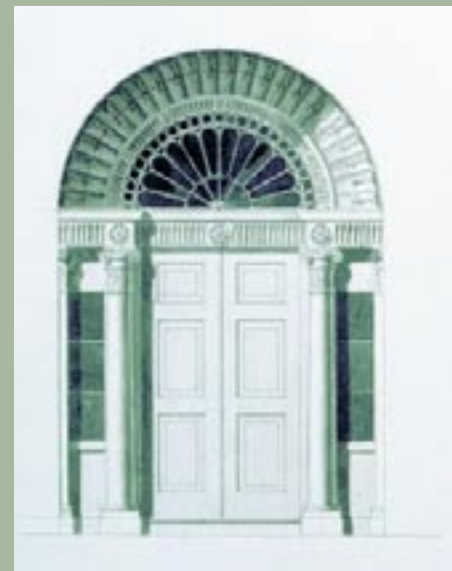
Doorcase design with Adamesque fanlight. Ink with grey and Indian ink washes, AD 2367.
